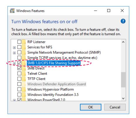
Once activated, we accept the changes and restart the computer. When it turns on again we will have SMB 1.0 working, and all the applications that depended on this protocol should work without problems equally in the last version of this operating system.
