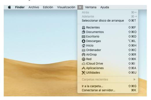
2 Enter smb:// x.x.x.x.x ,where x.x.x.x is the IP address of lightShark.
