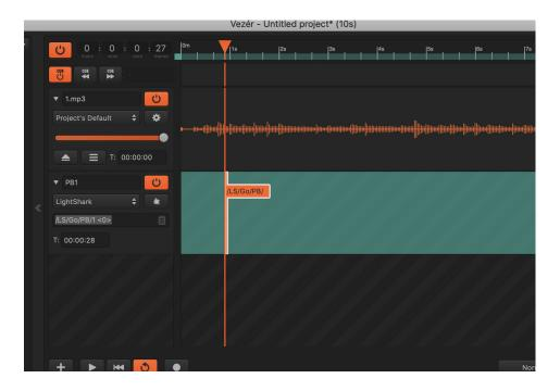
Note that actions in LightShark are performed by releasing the button, so the message is sent on <0> value instead of <1>.
