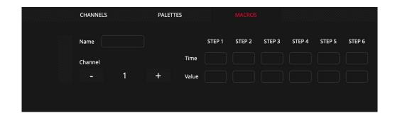
Press and hold the name field for two seconds to add a label to the Macro.
