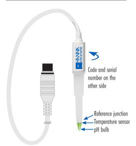
Quick connector with Rubber protection, and 1 meter cable
